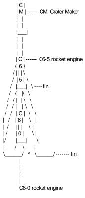
The fuse is put in the bottom engine.
